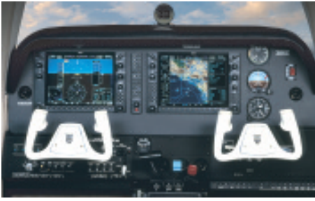
Garmin G1000 integrated avionics system.
